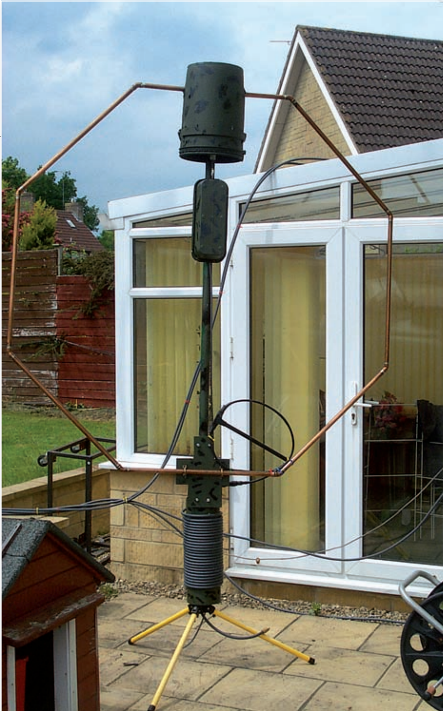
Fig. 1: General arrangement of the loop – with the balun acting as weight for stability.
