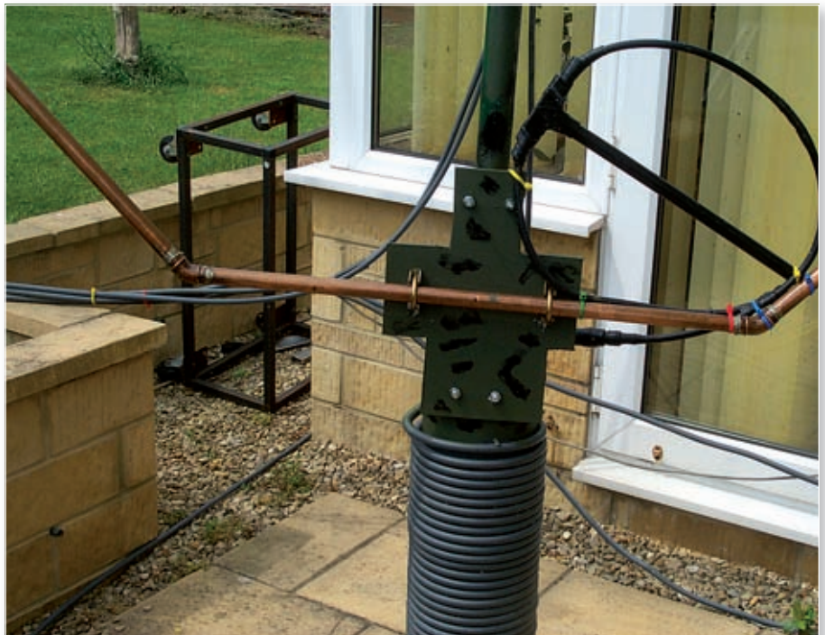
Fig. 3: The Faraday coupling loop (top right) – this should be positioned opposite the vacuum variable capacitor but it is not unduly critical.
